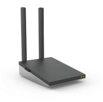
The **Fallback Module** is **available as an accessory** to the MC-X Dispatcher Console. The Fallback Module is used in situations where the Dispatcher Console is unable to establish a connection with the Dispatcher System Core. In this situation, the Fallback Module will ensure that the user can still communicate over the GSM-R network by establishing a direct communication link using the built-in **GSM-R Modem** and over the 4G/5G networks using the built-in **LTE Modem**.
